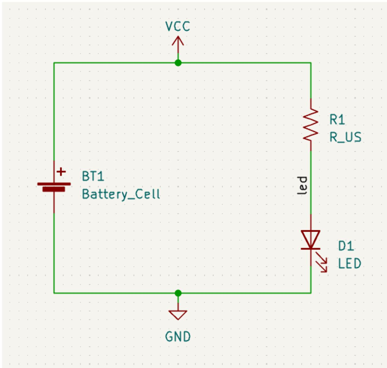
Note that labels and power symbols with the same name are connected together. Another GND symbol or wire labeled `led` on this schematic page would be shorted to the existing one, even without wires visually
