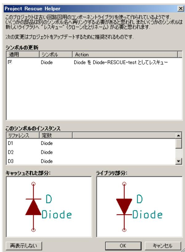
You can see in this example that the project originally used a diode with the cathode facing up, but the library now contains one with the cathode facing down. This change would break the schematic! Pressing OK
