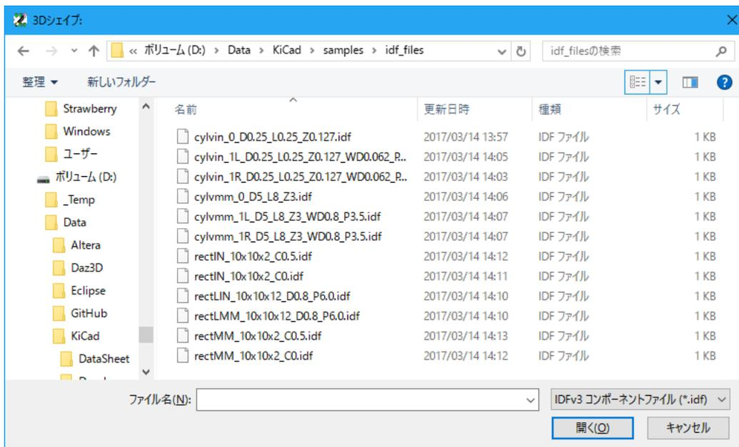
Once the desired component outline file is selected, enter any necessary values for the offset and rotation. The offsets must be specified using the IDF board output units (mm or mils) and in the IDF coordinate system, which is a right-hand coordinate system with +Z pointing towards the viewer, +X to the viewer's right, and +Y towards the upper edge of the screen. The rotation must be in degrees; positive rotation is a counter-clockwise rotation as described in the IDFv3 specification.
