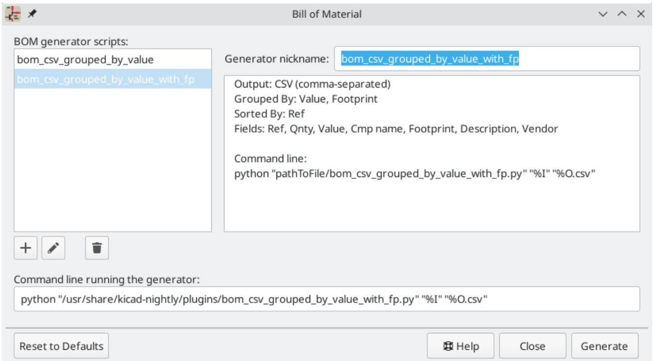
KiCad 7.0 uses Python scripts to generate BOMs. Three BOM scripts are included, and users can also create their own scripts to generate BOMs in whatever format is desired.
