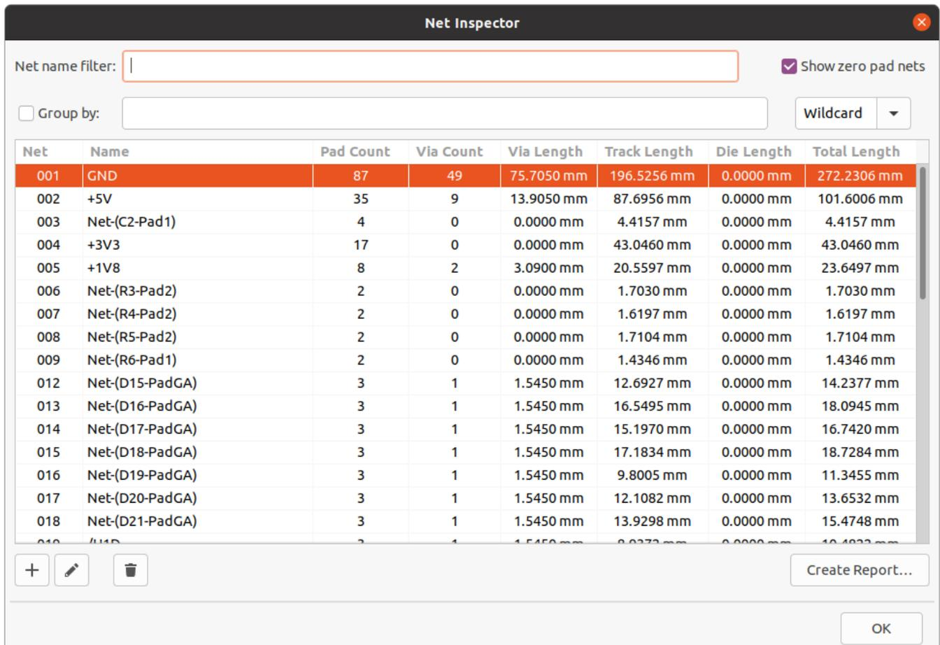
The screenshot shows the Net Inspector window with a table of net properties. The table has columns for Net, Name, Pad Count, Via Count, Via Length, Track Length, Die Length, and Total Length. The first row is highlighted in orange.
