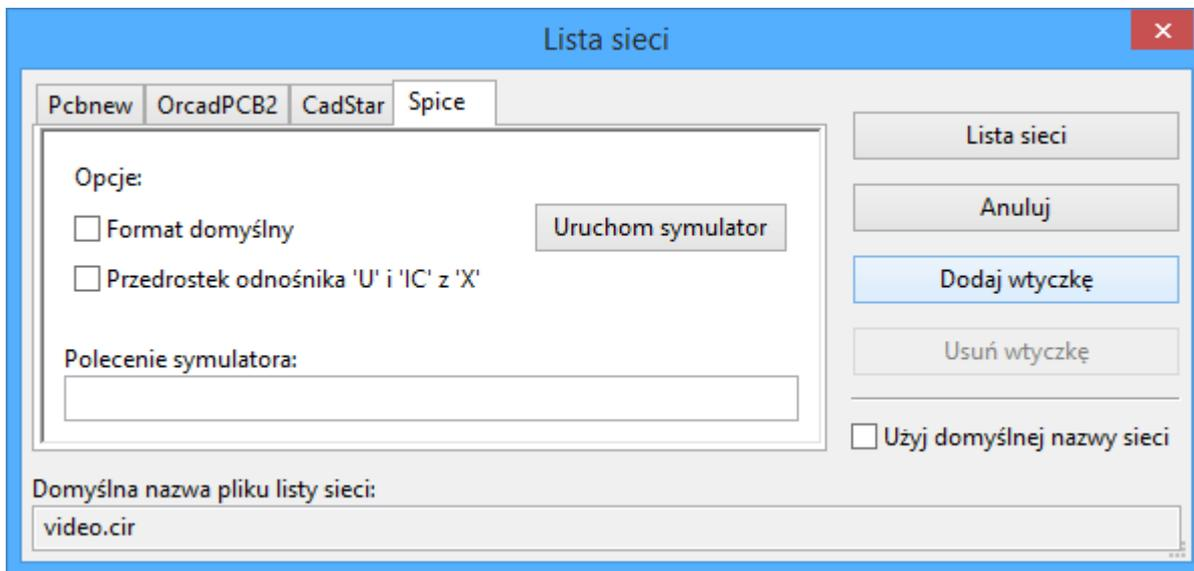
New generators require a name and a command. The name is shown in the tab label, and the command is run whenever the **Export Netlist** button is clicked.
