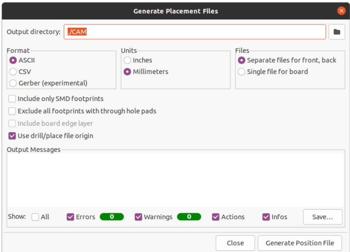
**Format:** Choose between generating a plain text (ASCII), comma-separated text (CSV), or Gerber placement file format.
